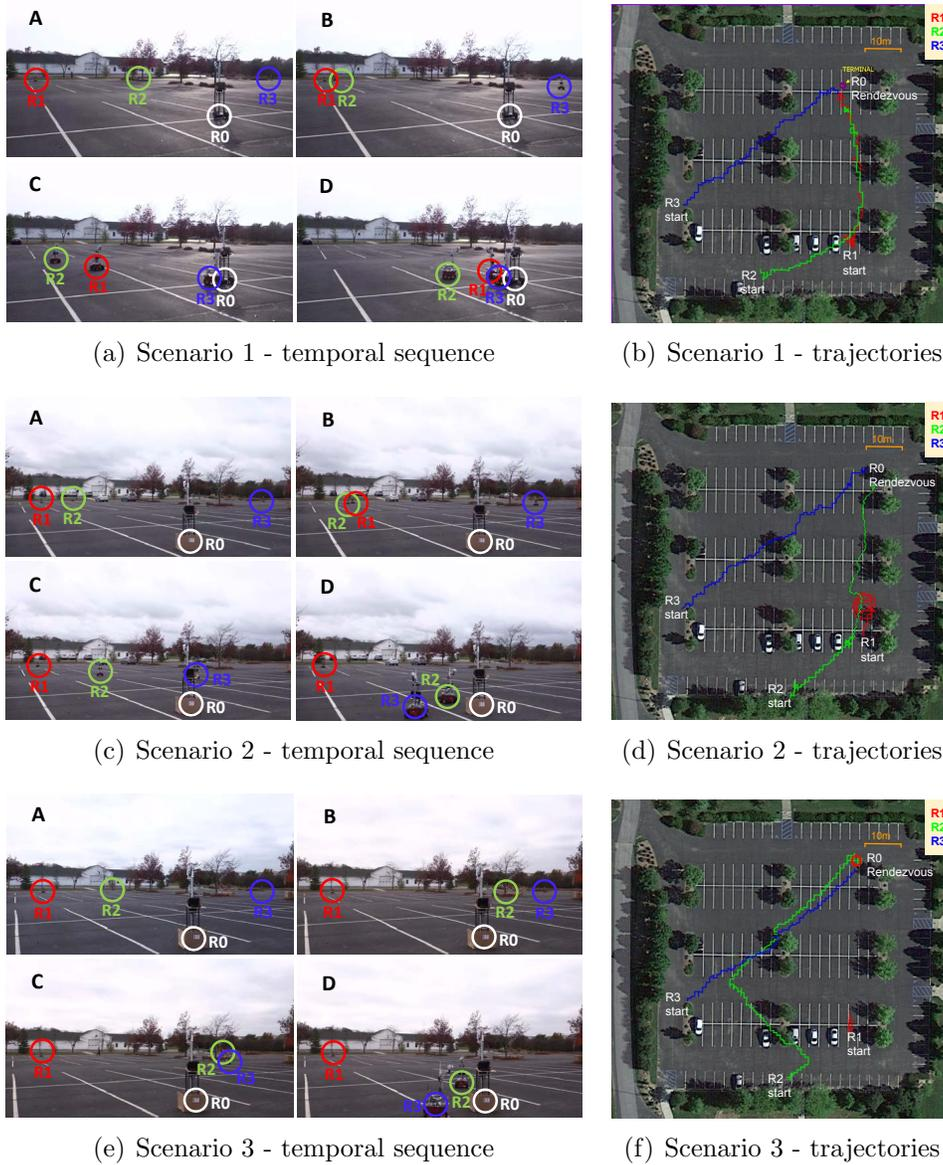
Figure 6: (a), (c), and (e) show a sequence of stills from experiments in Scenarios 1, 2, and 3. The temporal sequence is sorted alphabetically. (b), (d), and (e) are trajectories of the robots in Scenarios 1, 2, and 3 overlaid on the satellite image of the actual experimental site (a large and obstacle-filled parking lot). The trajectory of  $R_1$  is depicted in red, the trajectory of  $R_2$  is depicted in green, and the trajectory of  $R_3$  is depicted in blue.
