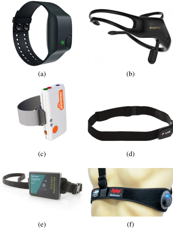
Fig. 3: A list of the biosensors that the proposed biosensor package currently supports; (a) Empatica E4-wristband [19], (b) EMOTIV Insight-5 Channel Mobile Brainwear [20], (c) Shimmer3 GSR+ Unit [21], (d) Polar H10-Heart rate monitor chest strap [21], (e) Vernier-Go Direct Respiration Belt [22], and (f) Zephyr BioHarness 3 [23]
